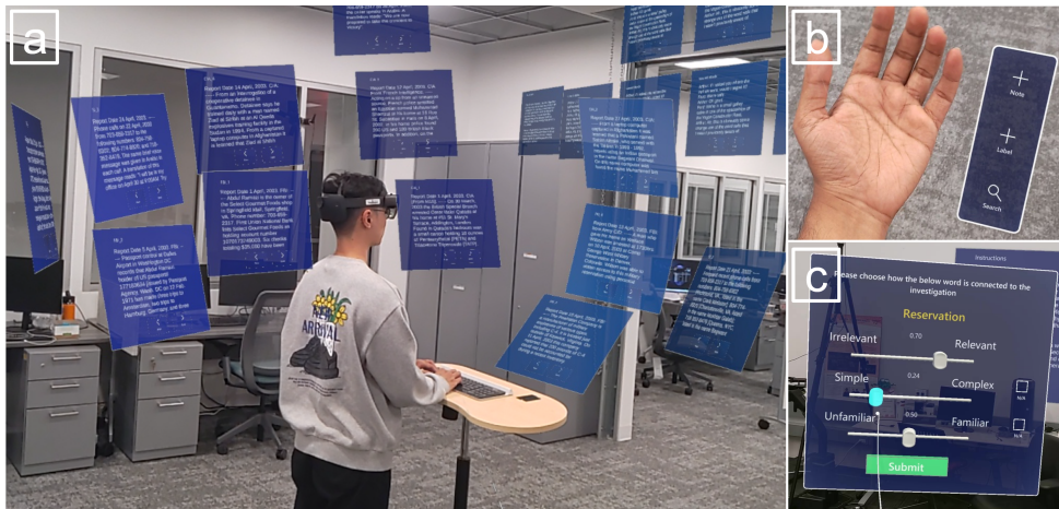
Figure 1: Overview of the EyeST prototype. a) An analyst views and interacts with text documents in Augmented Reality (AR) while eye-tracking data is collected. b) A hand-registered menu allows the analyst to annotate and search the dataset. c) The system retrieves a word that the analyst paid attention to, and the analyst rates it in terms of relevance, complexity, and familiarity.
