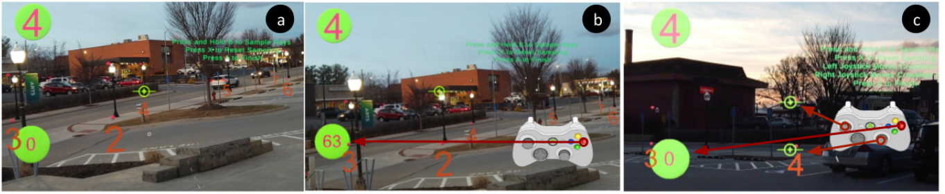
Fig. 4. The pointer's view using the pointing interface to specify: A single ray (a& b), and two rays (c). The number on the top left represents the target for the pointer. The number of samples taken by the pointer (ranging from 0 to 100) is shown on the bottom left.
