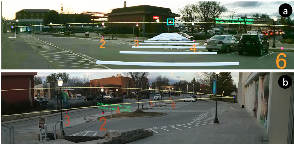
Fig. 1. Pointing Rays in AR 4. (a). Observer's view of the single ray marked by pointer aiming at Target 2, Parallel Bars are parallel to the single ray; the white sphere denotes the closest point on the ray to the observer (highlighted by blue square); (b). Observer's view of the Double Ray technique placed by the pointer aiming at Target 4; the two rays are visually bracketing the target lamppost. Images are captured from Microsoft HoloLens 2 and carry intrinsic offsets.
